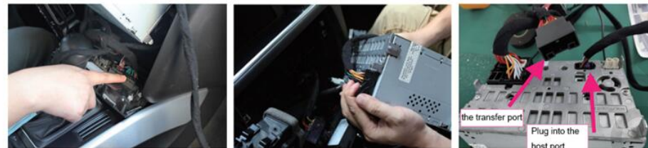
Complete the transfer of air conditioning panel
